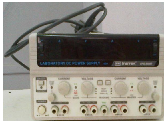
Figure 2: Laboratory DC power supply 4 channel
