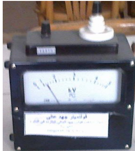
Figure 7 :High voltage Voltmeter 0:5 kv
