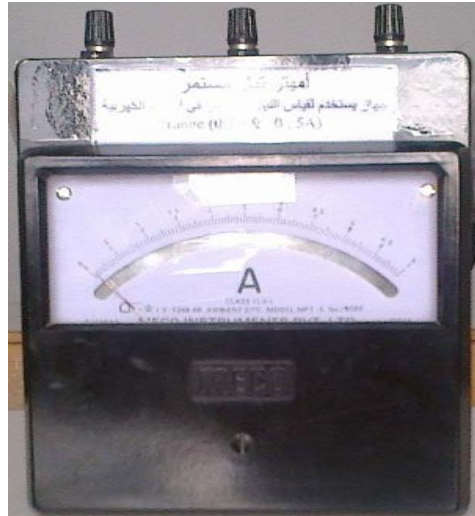
Figure 9 :AC Ammeter 0:5,0:10A
