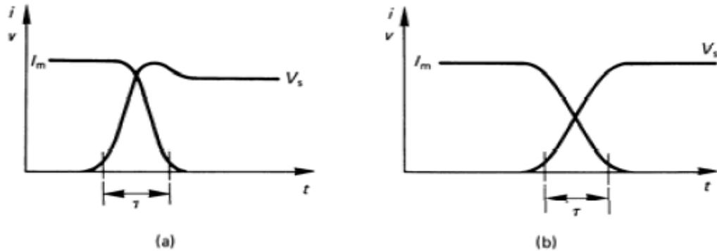
Figure 5.7. Typical voltage and current at turn-off switching transition for:
