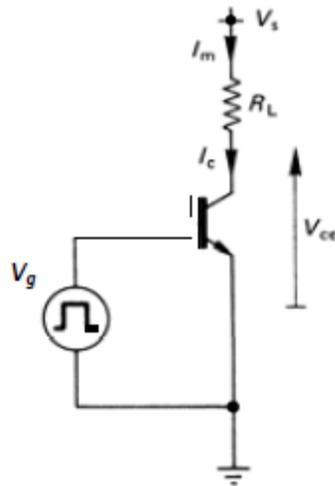
Figure 6.1. A typical IGBT transistor switching circuit incorporating a resistive load.
