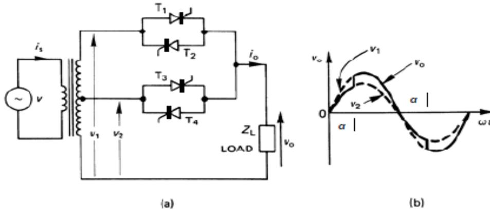
Figure 12.7. An ac voltage regulator using a tapped transformer: (a) circuit connection and (b) output voltage waveform with a resistive load.
