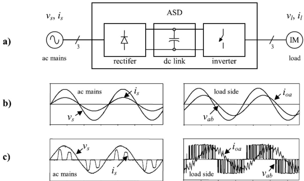
c- Design a three-phase PWM inverter that drives a 30hp, variable speed, 3-phase, 12-pole, 460V, 60Hz induction motor. The DC supply is 300V and  $m_a=0.8$  and  $m_f=15$ . Draw a block diagram of the system and use the following table to calculate the fundamental frequency line to line voltage and some dominant harmonics of line to line voltages.
