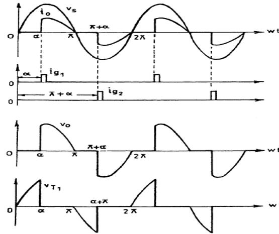
FIGURE 16.2 Waveforms for single-phase ac full-wave voltage controller with  $R$ -load.
