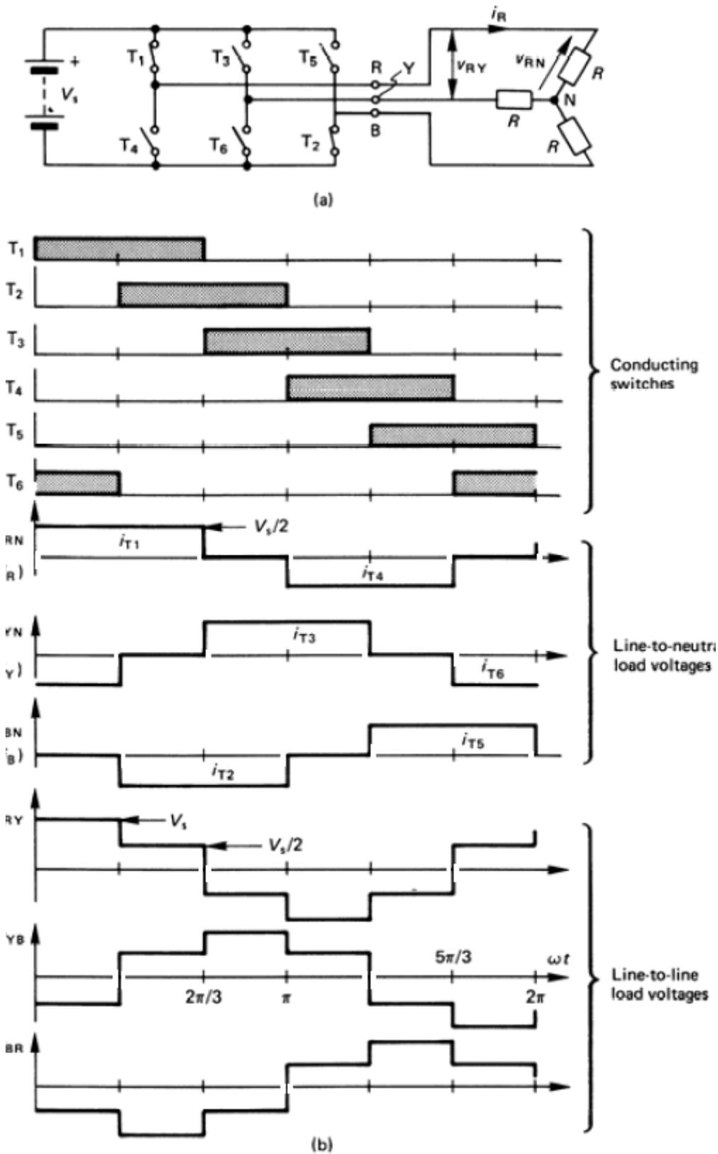
Figure 14.7. A three-phase bridge inverter employing 120° switch conduction with a resistive star load: (a) the bridge circuit showing  $T_1$  and  $T_2$  conducting and (b) circuit voltage and current waveforms.
