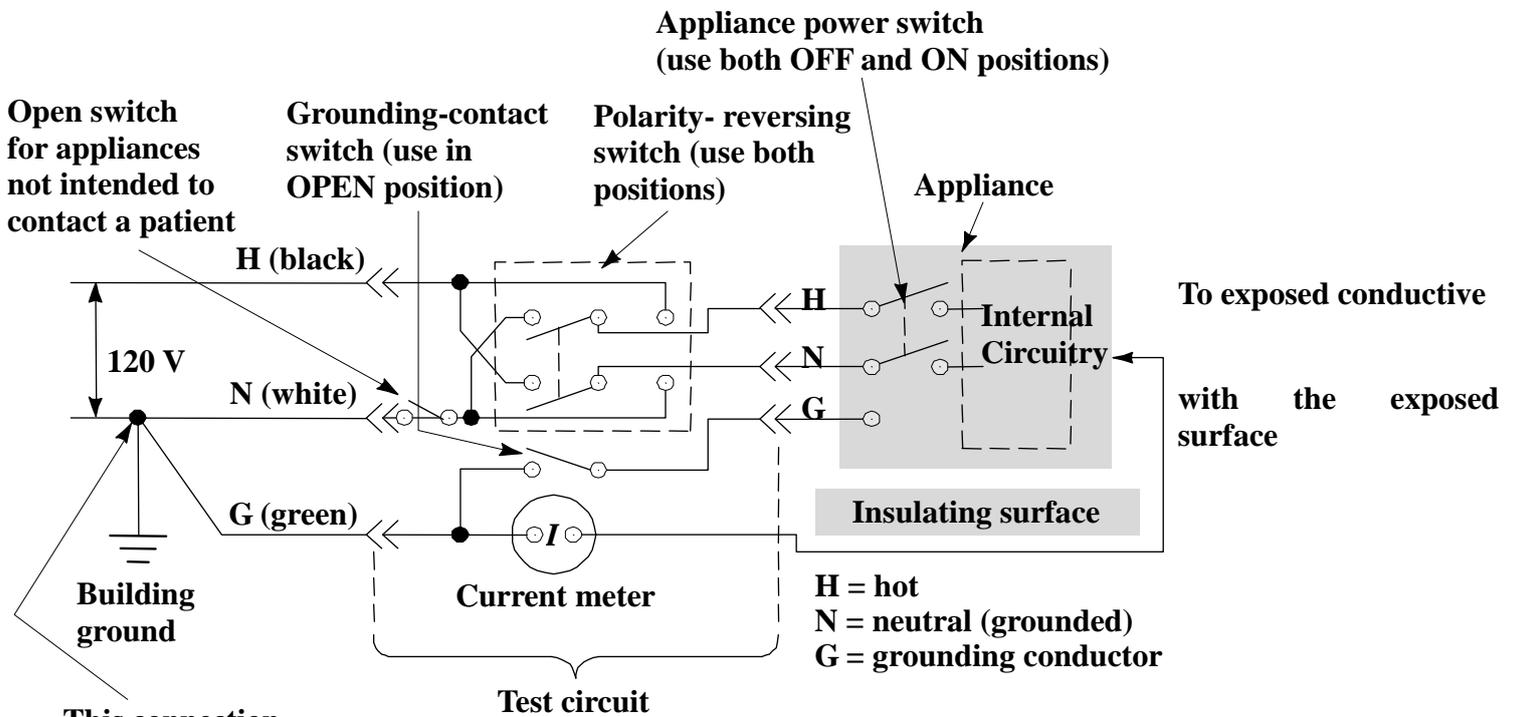
This connection is at service entrance or on supply side of separately derived system
