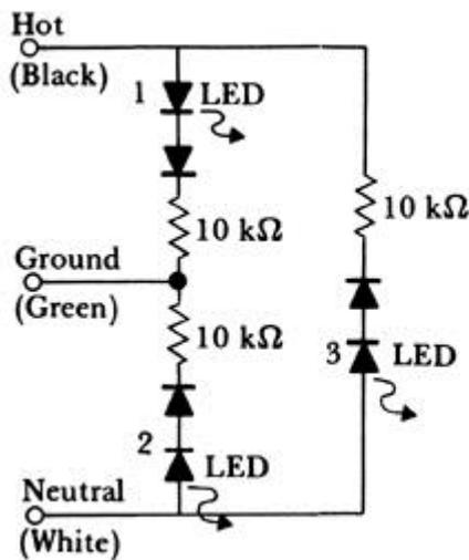
Wiring Codes ( \* ≡ LED on)
