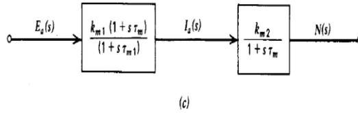
**Fig. 6.2** Development of motor transfer function. (a) Separately excited dc motor model. (b) Functional block diagram. (c) Simplified functional block diagram.
