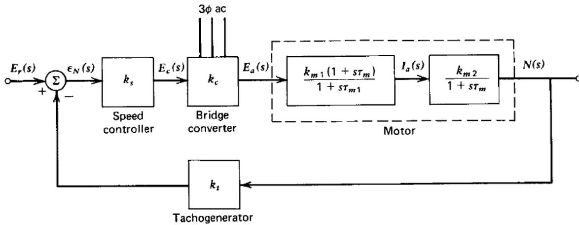
**Fig. 6.3** Speed-control loop.
