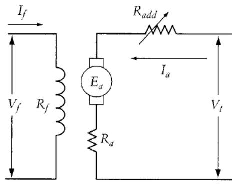
**Effect of adding an armature resistance on speed**
