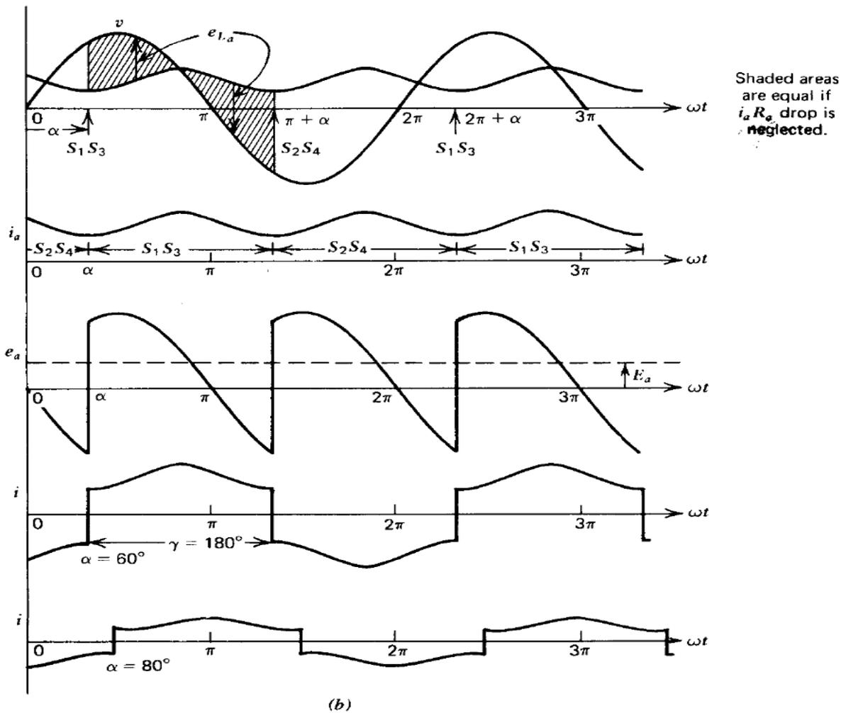
**Fig. 2.3** Speed control of a separately excited dc motor by a single-phase full-converter. (a) Power circuit. (b) Voltage and current waveforms for continuous motor current (motor operation). (c) Waveforms for inversion operation.
