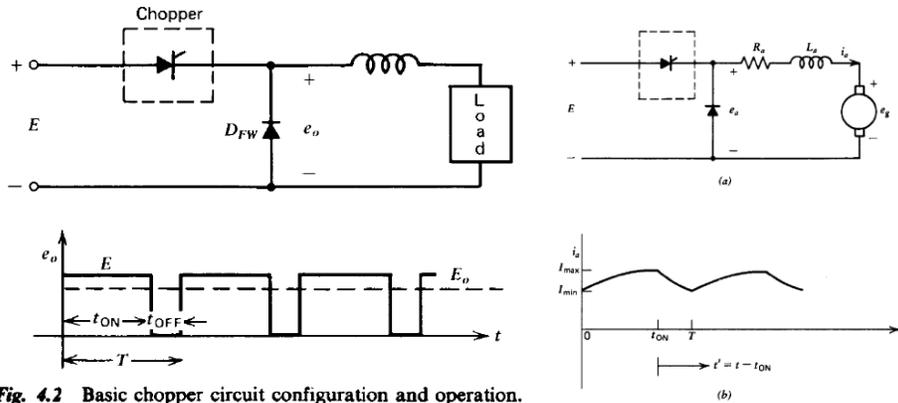
Fig. 4.2 Basic chopper circuit configuration and operation.
