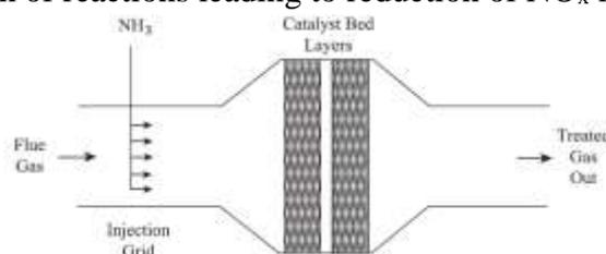
SCR systems are capable of reducing NO<sub>x</sub> up to 90%. In the common power- generation application of gas-fired turbines, less than 5 ppm NO<sub>x</sub> at 15% O<sub>2</sub> can be achieved.
