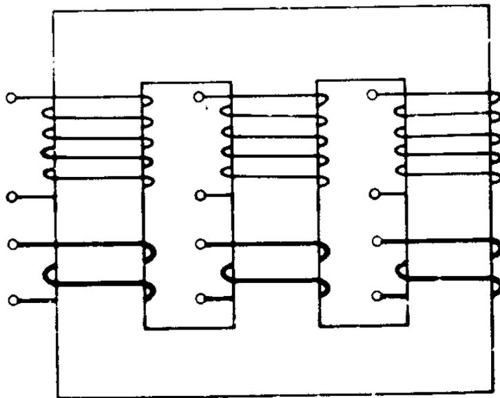
FIGURE 3-14 Basic construction of  $\phi$ -phase transformers: (a) shell type;
