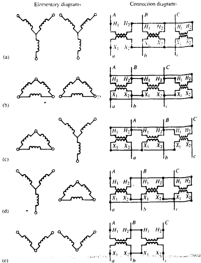
FIGURE 3-12 Three-phase connections of single-phase transformers.
