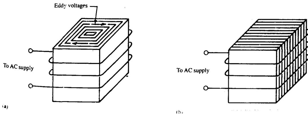
Figure 1-15 currents in solid iron core; (b) laminated core.
