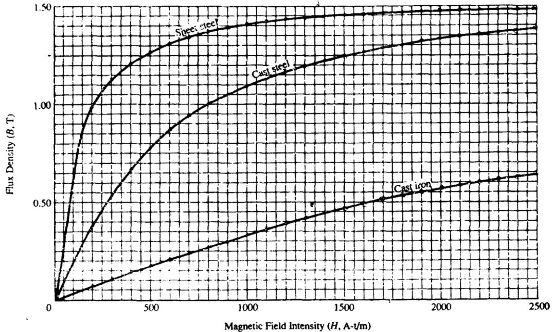
**FIGURE 1-3 Representative B-H curves for some commonly used ferromagnetic materials.**
