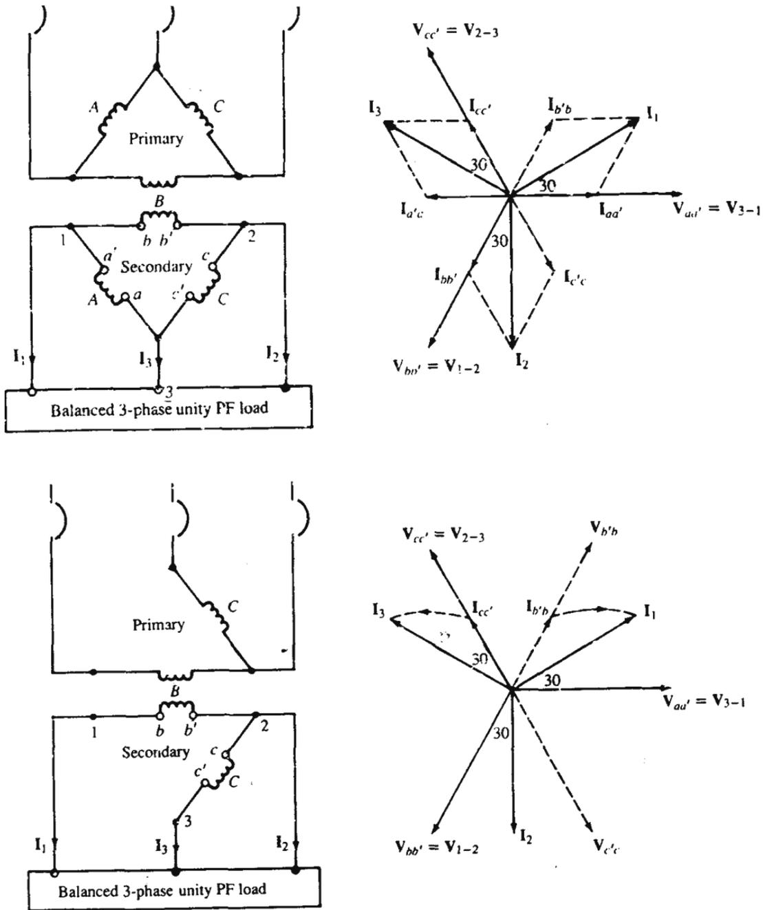
FIGURE 3-13 (a) Delta-delta bank; (b) phasor diagram for (a); (c) V-V bank; (d) phasor diagram for (c).
