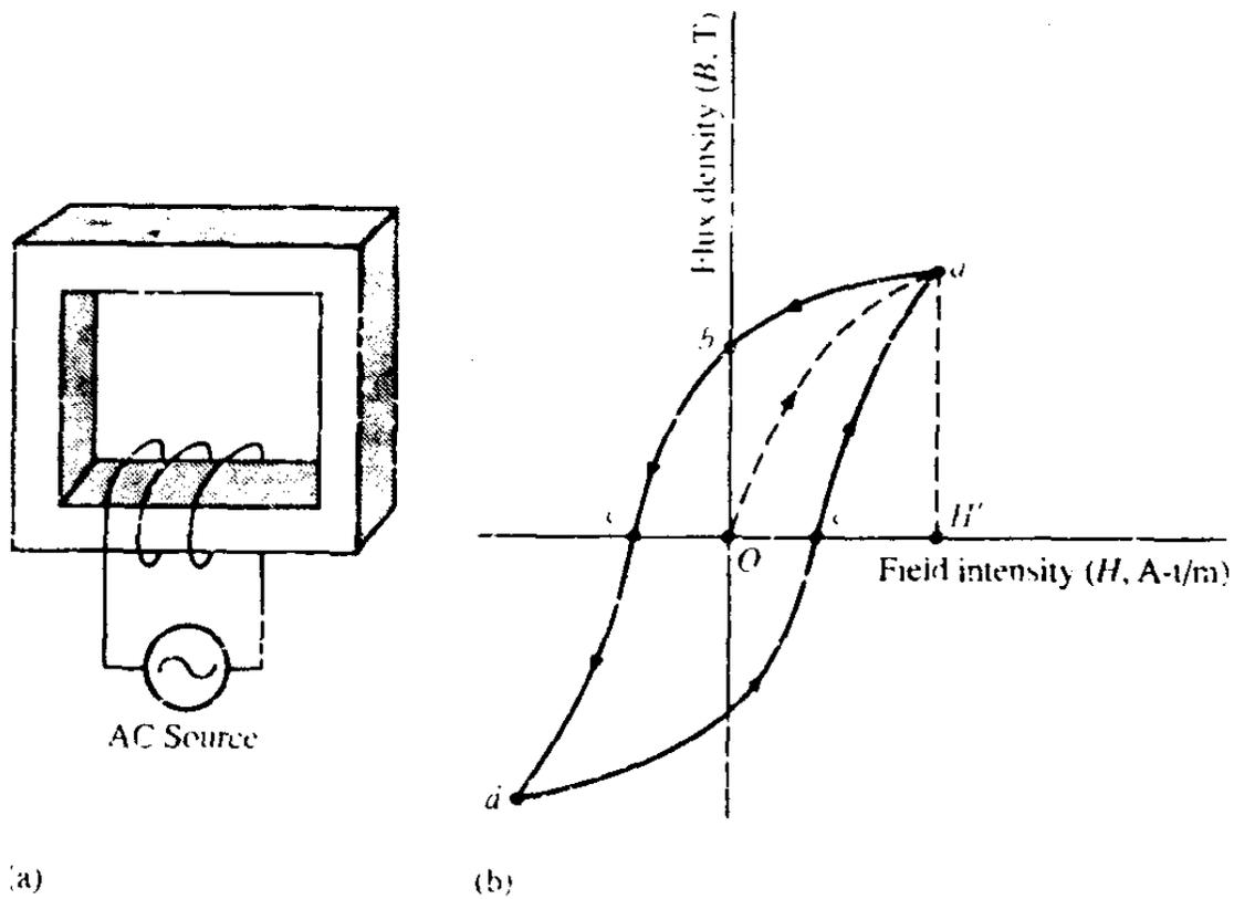
FIGURE 1-8 (a) Magnetic circuit with an alternating mmf:
