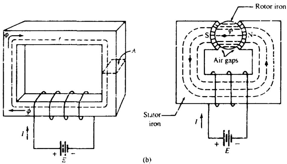
FIGURE 1-2 Magnetic circuit: (a) for a transformer;
