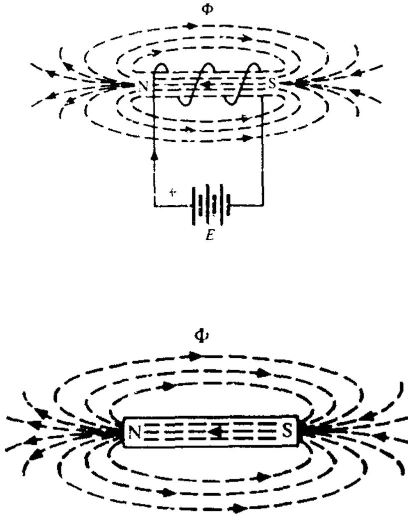
FIGURE 1-1 Direction of magnetic flux: (a) around a current-carrying conductor; (b) in a coil; (c) about a magnet.
