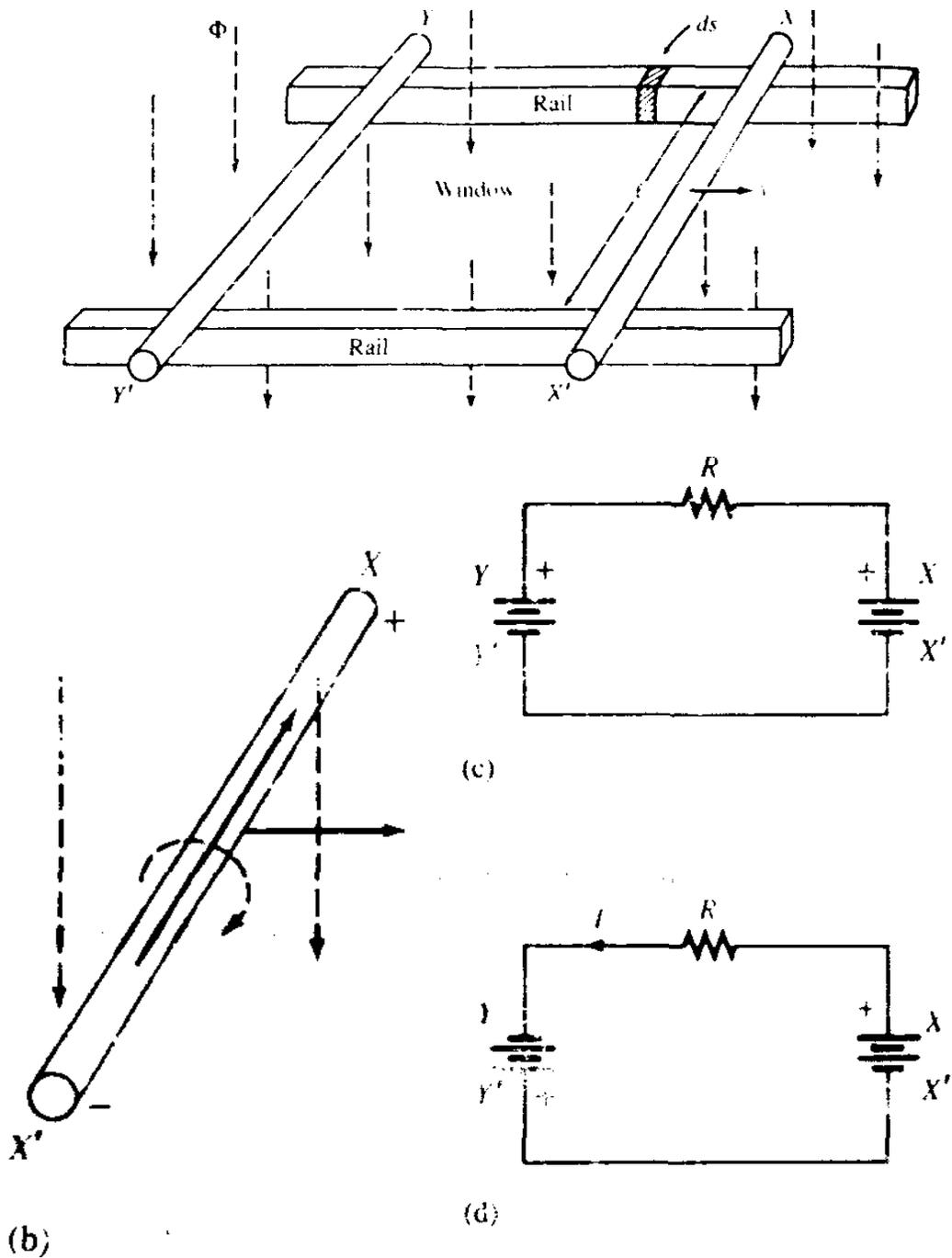
FIGURE 1-13 Closed loop consisting of two conductors and a set of conducting rails; (b) direction of emf and current caused by conductor moving to the right; (c) equivalent circuit, both conductors moving in the same direction; (d) equivalent circuit, conductors moving in opposite directions.
