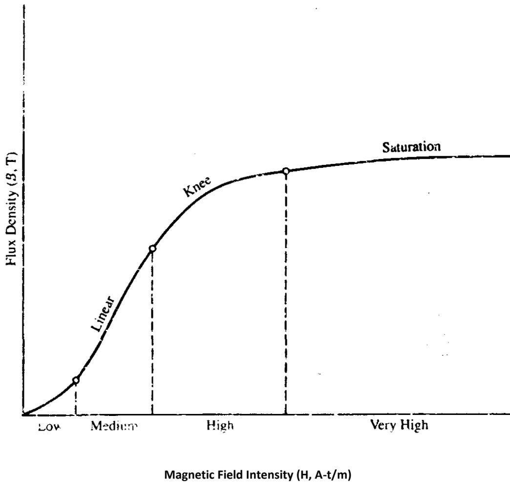
FIGURE 1-4 Exaggerated magnetization curve illustrating the four principal sections.
