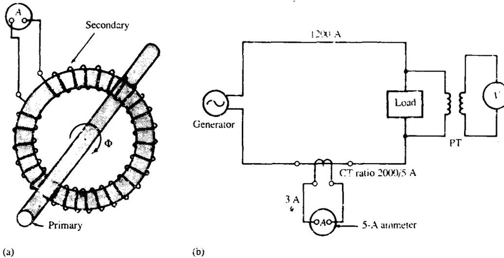
Figure 3-18 Current transformer; (a) window type; (b) circuit connections.
