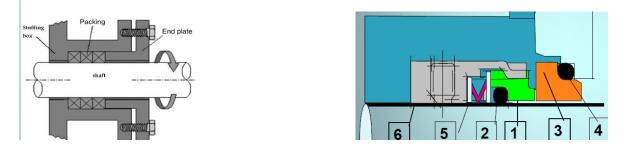
1.4) advantage of used packing 1)- This is a simple 2) - low cost, and easy to maintain 3) - Controlled leakage by tighten the gland 1.5)
