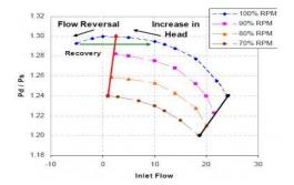
**Stalling** is the separation of flow from the compressor blade surface Types of stalling
