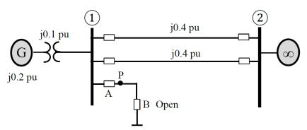
(b) Calculate the critical clearing angle and the critical clearing time for the system shown in the figure when the system is subjected to a three-phase fault at point P on the short transmission line.
